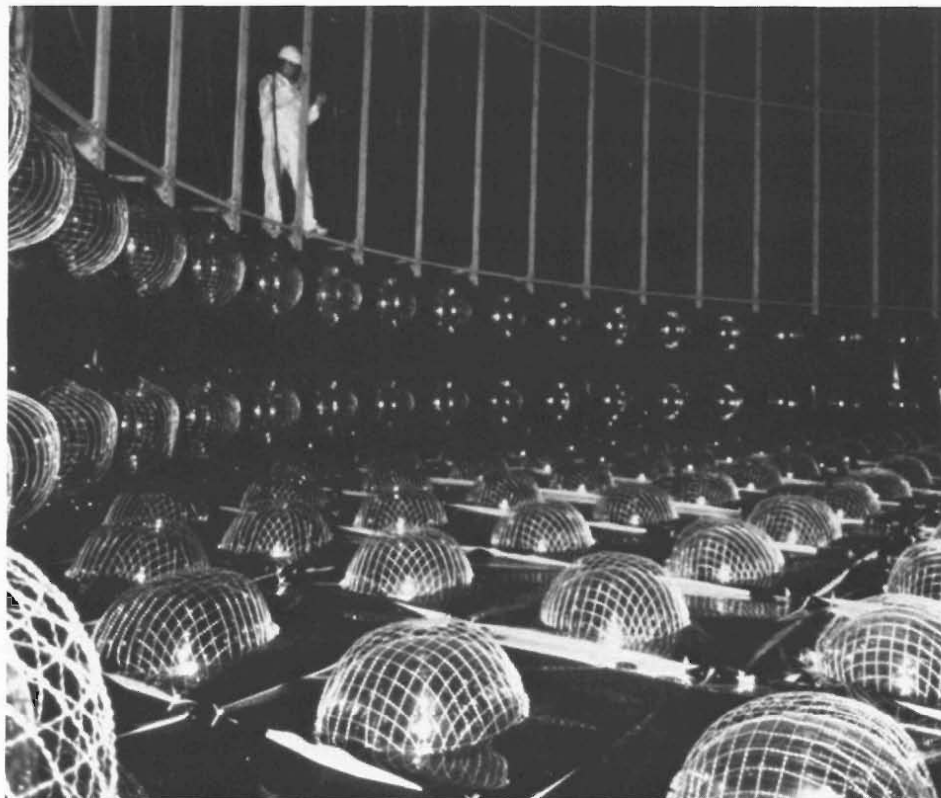
Fig. 3. Photograph of the Kamioka nucleon-decay detector under construction at a depth of 2700 mwe in a lead-zinc mine about 300 kilometers west of Tokyo. Already installed are the bottom layer of photomultipliers and two ranks of photomultipliers on the sides of the cylindrical volume. The wire guards around the photomultipliers protect the workers from occasional implosions. The upper ranks and top layer of photomultipliers were installed from rafts as the water level was increased. The detector contains a total of 1000 20-inch photomultipliers. (Photo courtesy of the Kamioka collaboration.)
